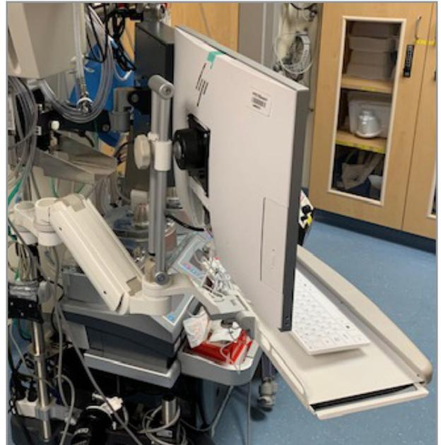
The mobile cardiopulmonary bypass machine cart above features ICWUSA's patented Ultra 180 arm and pole mount which help support the computer and keyboard workstation. The workstation also features the KUB keyboard, which has an ergonomic poly wrist rest.
