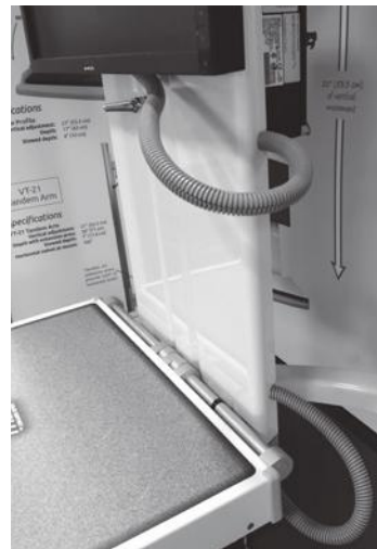
Wire management showing split wire loom.
