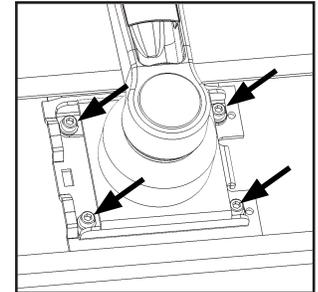
Using the four screws and lock washers removed in step 1, install the Slider Mount Assembly.
