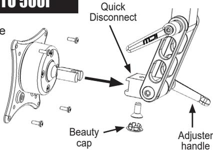
Slide VESA assembly into Quick Disconnect. Tighten screw with 5/16" hex key. Replace beauty cap.
