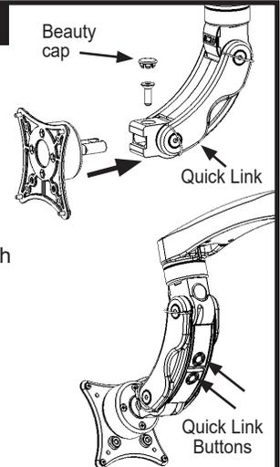
Adjust monitor height and angle by pressing buttons on Quick Link. Move monitor to desired position and release buttons.
