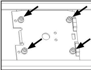
Remove the four socket head cap screws and lock washers located on the track.
