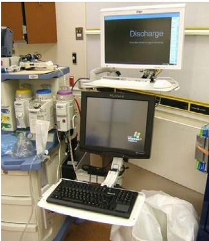
Anesthesia cart with dual monitors, scanner and service tray mounted on a pair of ICW's heavy duty Titan Arms. This configuration provides a complete workstation and stows compactly.
