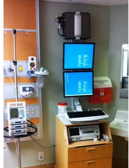
*(Top) Dual monitors and frame-mounted CPU mounted used with a fetal monitor cart. (Bottom) MD Arm with Paralink, monitor and keyboard mounted on a Draeger anesthesia cart.*
