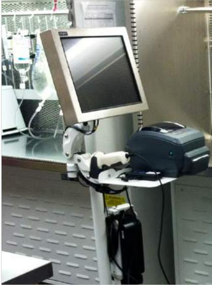
*Ultra Pole Mount configuration for a Baxter DoseEdge Medication Delivery System in a pharmacy clean room. The mount holds a touchscreen monitor with scanner and Zebra printer.*
