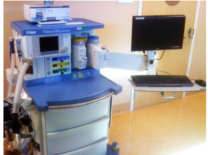
MD Arm with Paralink, monitor and keyboard on a Draeger anesthesia cart.
