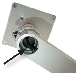
Wires run through the joints.
