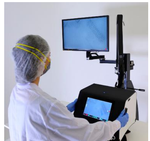
After positioning the ML-Pro Crime Lite®, the Elite 5216 arm's internal gas springs allow the user to keep the device level and stable, despite its bulk.
