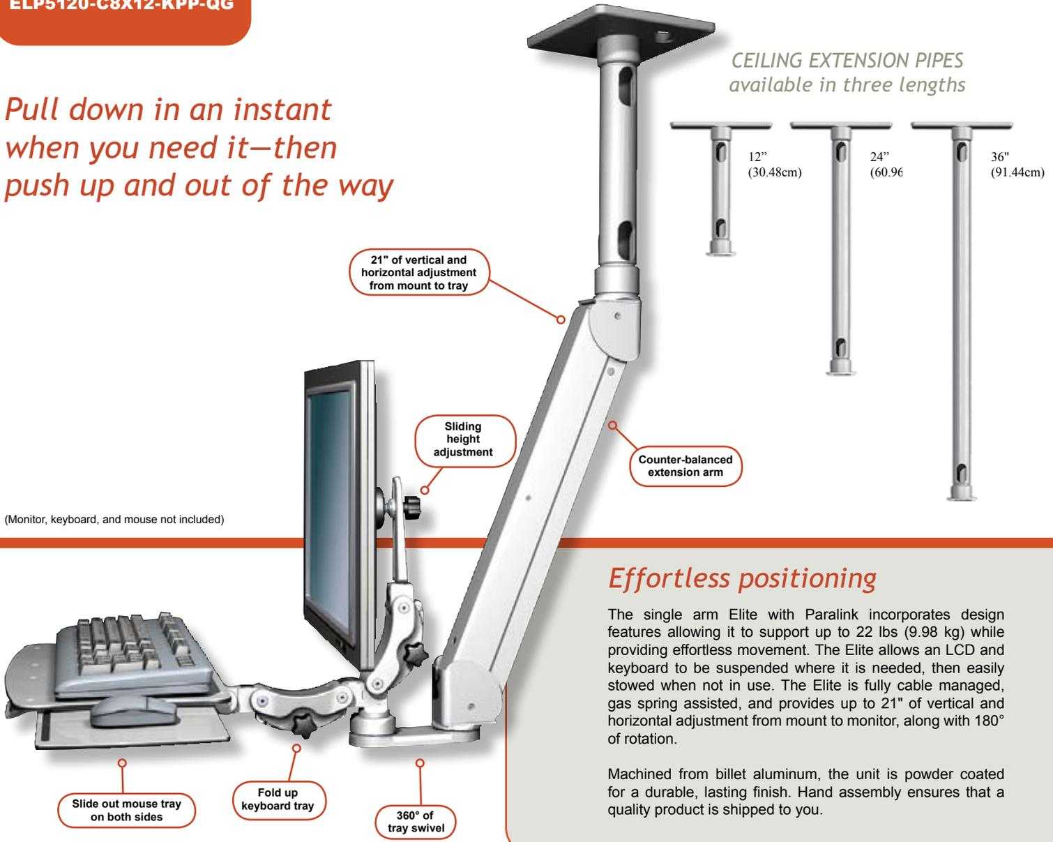
CEILING EXTENSION PIPES available in three lengths
