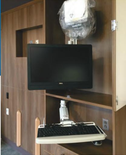
*Above the shelf, an Inverted Ultra 180 with two AS1 extensions hold the monitor and a Mini-PC. Below the shelf at the rear of the cabinet, a second Inverted Ultra 180 with one AS1 extension hold the keyboard tray.*
