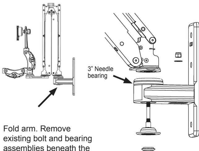
Fold arm. Remove existing bolt and bearing assemblies beneath the wall ear. Replace with new hardware provided.
