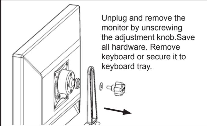
Unplug and remove the monitor by unscrewing the adjustment knob. Save all hardware. Remove keyboard or secure it to keyboard tray.
