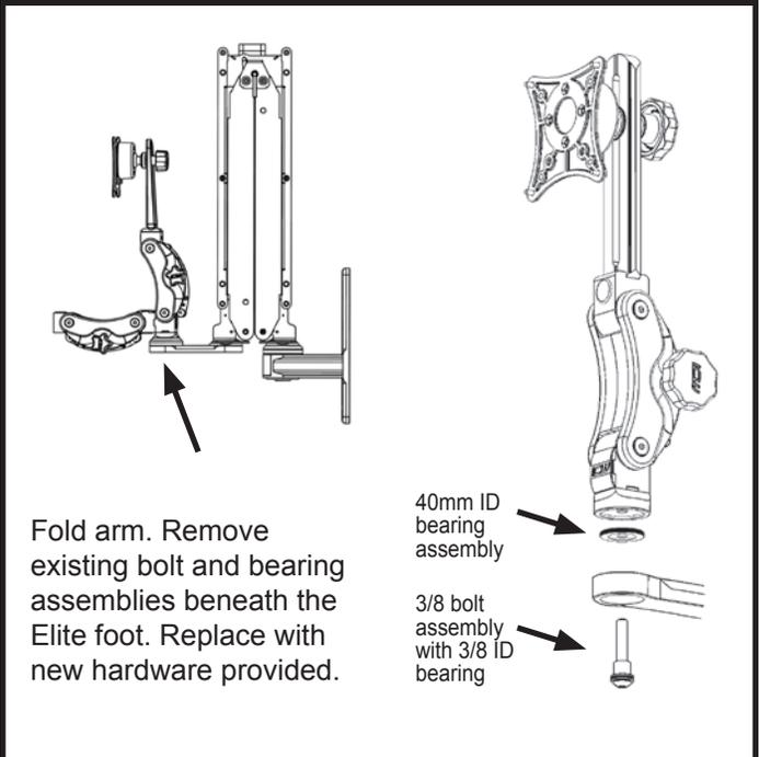
Fold arm. Remove existing bolt and bearing assemblies beneath the Elite foot. Replace with new hardware provided.
