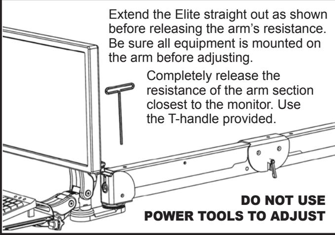
Extend the Elite straight out as shown before releasing the arm's resistance. Be sure all equipment is mounted on the arm before adjusting.
