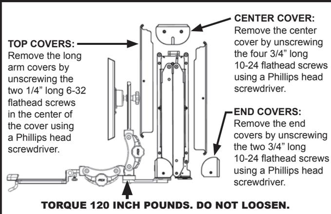
**TOP COVERS:** Remove the long arm covers by unscrewing the two 1/4" long 6-32 flathead screws in the center of the cover using a Phillips head screwdriver.
