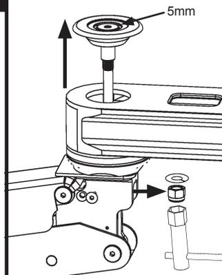
Remove end cover on end of Elite Arm under wall ear. Loosen 3/8 bolt with provided 5mm hex key while using provided 9/16 wrench to hold nylock nut as you loosen 3/8 bolt.
