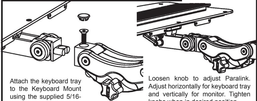
Loosen knob to adjust Paralink. Adjust horizontally for keyboard tray and vertically for monitor. Tighten knobs when in desired position.
