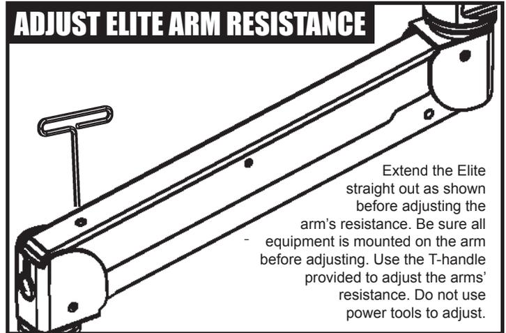
Extend the Elite straight out as shown before adjusting the arm's resistance. Be sure all equipment is mounted on the arm before adjusting. Use the T-handle provided to adjust the arms' resistance. Do not use power tools to adjust.
