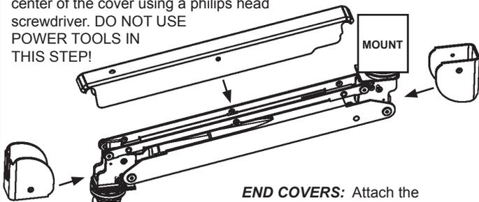
**END COVERS:** Attach the end covers by screwing the two 10-24 flathead screws using the 1/8" hex key. **DO NOT USE POWER TOOLS IN THIS STEP!**
