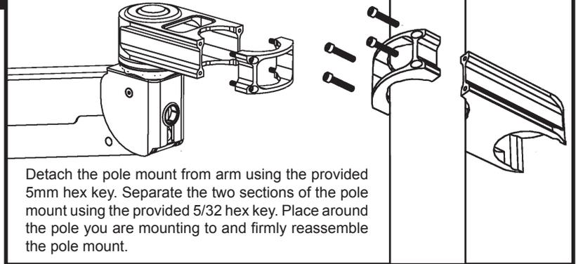
Detach the pole mount from arm using the provided 5mm hex key. Separate the two sections of the pole mount using the provided 5/32 hex key. Place around the pole you are mounting to and firmly reassemble the pole mount.
