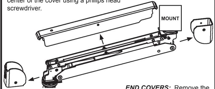
**END COVERS:** Remove the end covers by unscrewing the two 10-24 flathead screws using the 1/8" hex key.
