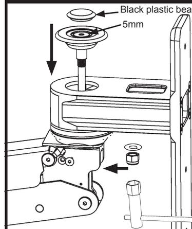
Pass 3/8 bolt with bearing assembly through wall mount ear and into end of Elite Arm. Secure Elite Arm under wall mount using split lock washer and nylock nut with 9/16 wrench provided and 5mm hex key.
