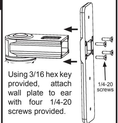
Using 3/16 hex key provided, attach wall plate to ear with four 1/4-20 screws provided.
