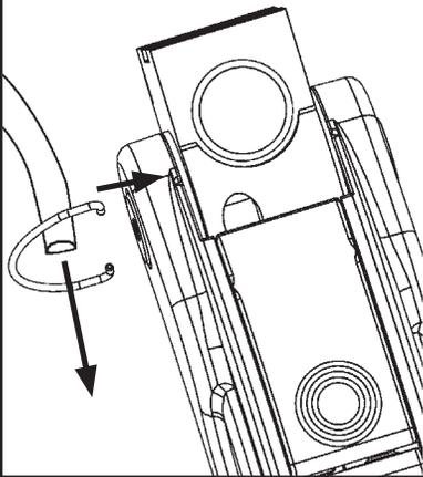
**NOTE:** The two clips provided can be installed on either side as needed.
